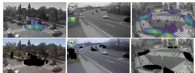
Figure 3: (Top) Heatmap measuring the maximum time any object spent in each pixel, normalized to the max (yellow) per video. (Bottom) The resulting masks used for our evaluation, chosen from the list of masks automatically generated using the algorithm in §I of [33].
