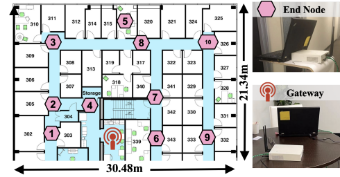
Figure 19: The indoor experimental plan and SDR devices spread out across tens of rooms.
