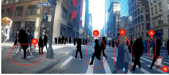
Figure 1: A video clip after (silhouette) denaturing exemplifying some of its shortcomings: (A) entirely missed detections, (B) potentially-identifying objects not incorporated in privacy definition, (C) silhouette may reveal gait.
