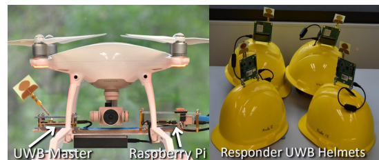
Figure 1: Left: The TrackIO setup with a DJI Phantom 4 UAV carrying a master UWB node and the Raspberry Pi controller units, Right: 4 UWB equipped helmets for first responders.
