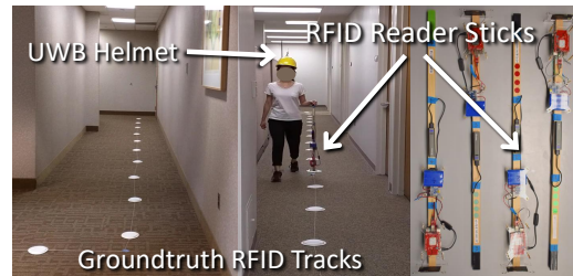
Figure 15: Snapshots of trajectories marked with RFID tags. A volunteer is shown walking along the track with the RFID reader stick in her hand.
