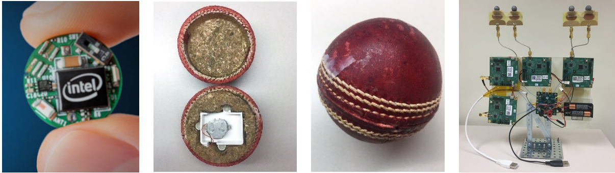
Figure 2: Ball instrumentation: (a) Intel Curie board with IMU sensors and UWB radio. (b) Scooped out cricket ball for snug fit of the sensor box. (c) Closed ball with sensor box. (d) UWB 4-antenna MIMO radio serving as an anchor.
