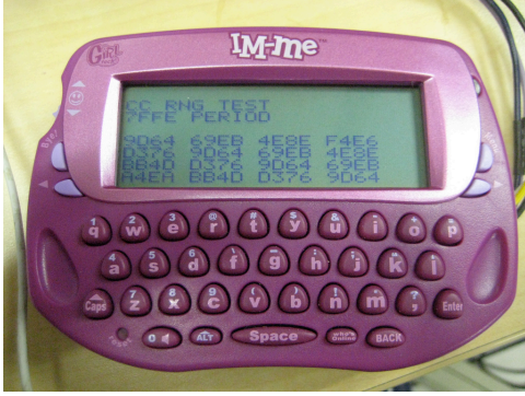
Figure 7: Girltech IMME, with modified firmware
