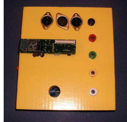
Figure 5: The mounting board for a single component. It contains three serial ports (along the top), 4 GPIO pins and a ground pin (along the right side), as well as a gumstix processor board mounted atop an expansion board.
