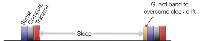
Figure 1: Minimizing guard bands reduces wasted active time and increases channel capacity.
