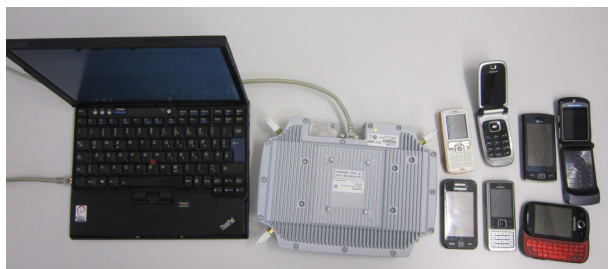
Figure 1: Our setup: A laptop that runs OpenBSC and the fuzzing tools, the nanoBTS, and some of the phones we analyzed.
