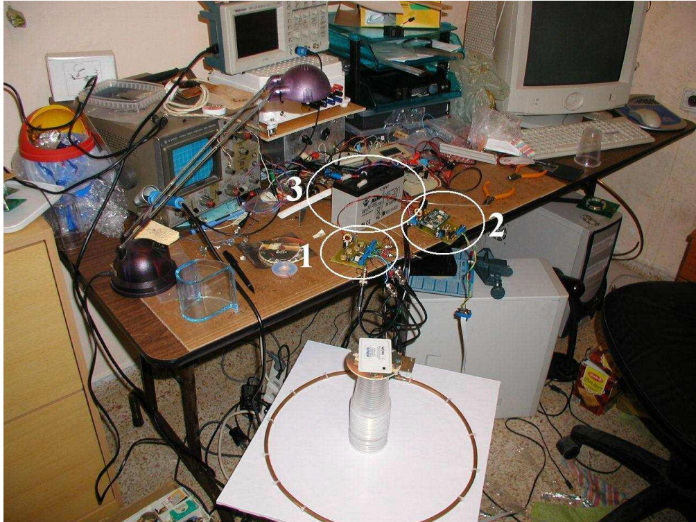
Figure 12: The antenna tuning process. Note the tag placed over a stack of plastic cups and beer coasters in the center of the antenna. The power amplifier is marked as item 1, the reader base board is marked as item 2 and the battery is marked as item 3.
